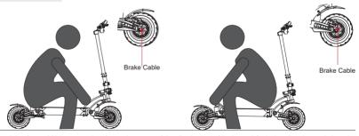
If the brake is too tight,pls use M5 hex wrench to loose the screw of the disc brake holder by anticlockwise direction,and short the brake cable,then fix the screw tightly; if the brake is too loose, just loose the screw and make the brake cable to be longer and then fix the screw tightly.
