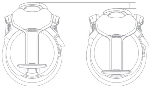
**Trolley Handle:** Press the unlock button under the Trolley handle to unfold it; when the Trolley handle is not in use, hold the lock button under the Trolley handle to fold.
