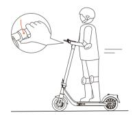
3. Stand on the footrest with both feet, press the throttle on the right hand. Note: For your safety, the motor will not engage until the scooter reaches 3 km/h.
